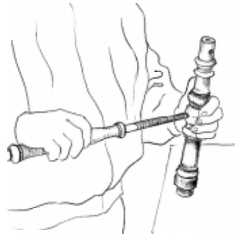
Step 4: Screw wheel adjusting screws (2) in to wheel posts (2); you will need to go all the way to the end. The screw starts on the same side as the small hole at bottom of the post.
